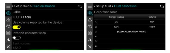
Some fluid level devices are reporting volume capacity by themselves. Use option "Use volume reported by the device" to automatically read tank capacity from device.
