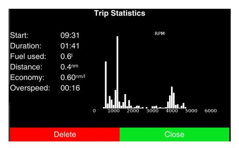
Start of current trip and its duration. Duration is taking into account only time, when engine was running. Fuel used during trip. Distance covered. Fuel Economy, which is calculated based on distance covered and fuel used during duration of this distance being done.
