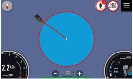
If compass is presented on NMEA2000 network, orientation of vessel is based on compass heading, otherwise vessel is always pointing towards anchor position.
