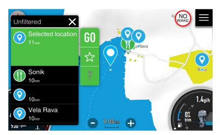
Header row indicates which filter is used for points. Press it to change filter. Press X to close dialog.
