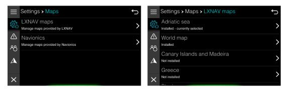
A list of all available maps data is shown together with indication, if it is installed or not. Selected item you would to manage. A new screen will open as shown on picture below.
