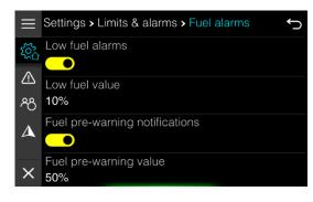
For fuel you have also two stage warning system. Fuel pre-warning value will generate informational warning (white). Low fuel value will generate important warning.
