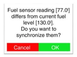
Calculated fuel and measured fuel are both shown od dashboard screens, fluid screen and chart screen. User can also set a floating box with both values.
