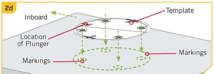
**NOTICE:** Drill the holes for the screws completely through to prevent splitting the boat deck.
