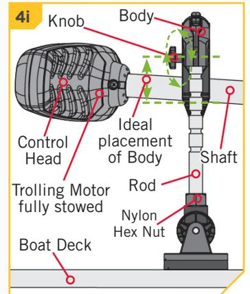
**NOTICE:** When cutting the Rod at least one notch on the Rod must remain. If unsure, leave the Rod longer, and cut off fewer notches and test after each notch is removed before finishing the installation, or have the bracket installed by a qualified marine installer.
