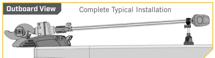
3. The base of the bracket includes a Plunger that is used to adjust the Swivel Base of the bracket. The Swivel Base can be locked into 7 positions by pulling out the Plunger and rotating it up to 180 degrees at 30 degree increments.
