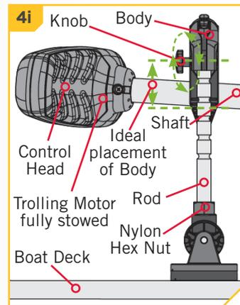
**NOTICE:** When cutting the Rod at least one notch on the Rod must remain. If unsure, leave the Rod longer, and cut off fewer notches and test after each notch is removed before finishing the installation, or have the bracket installed by a qualified marine installer.
