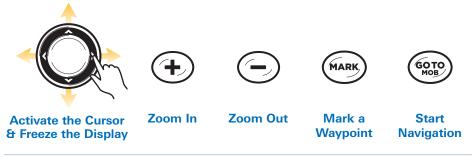
**NOTE:** If your unit does not have ZOOM keys, move the cursor, and open the Down Imaging X-Press Menu (Custom) > DI Zoom to adjust the magnification.
