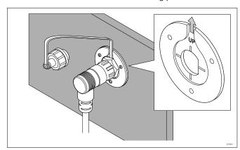
To ensure that the handset's connector points down when connected, orientate the mounting plate so that the lanyard grove is pointing straight up.
