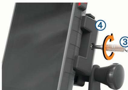
**NOTE:** The security screw is used to deter device theft and helps prevent you from accidentally pressing the release latch.
