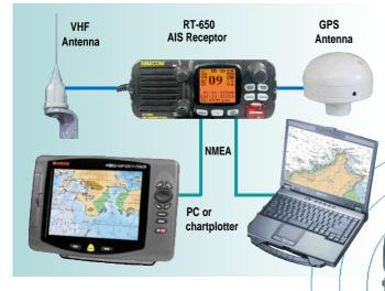
Only one antenna for the CHF transmission and the AIS system.
