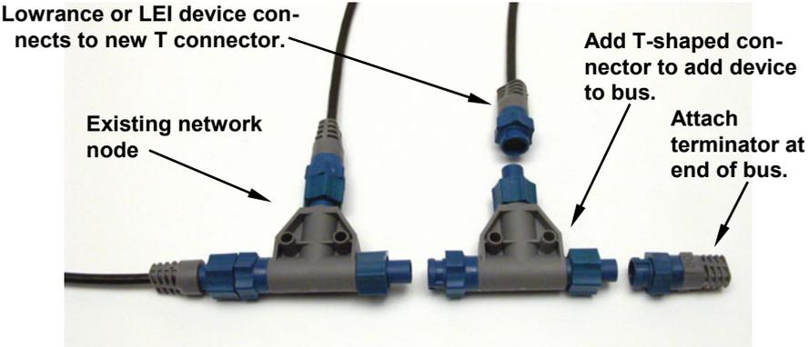
Add a new device to a NMEA 2000 bus (above) by attaching a T connector between two T connectors, between a T connector and the end terminator, or between two backbone extension cables. The red connector network (below) is built in the same way. Notice the Double T connectors on the red connector network.
