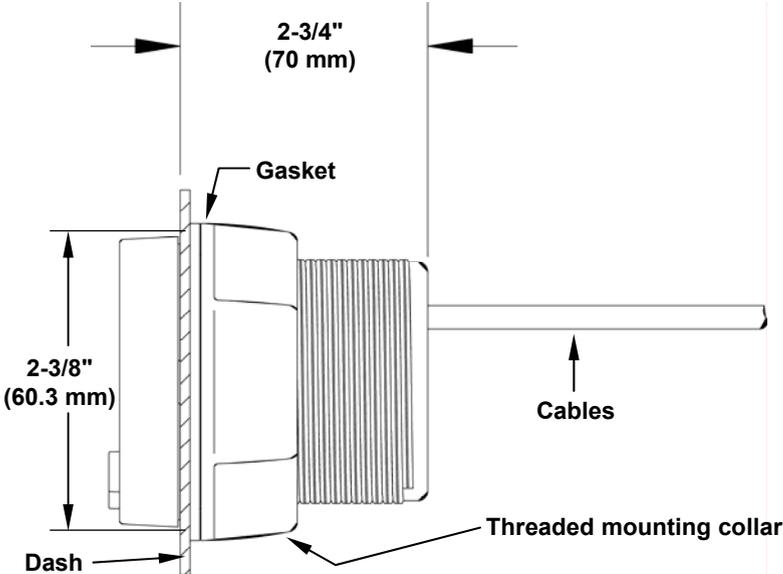
Dash installation, cross-section view.
