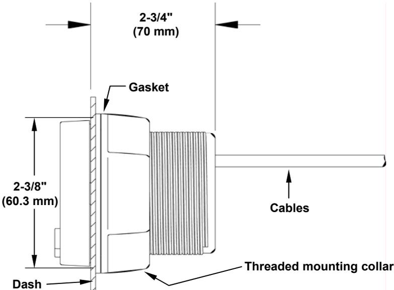
Dash installation, cross-section view.
