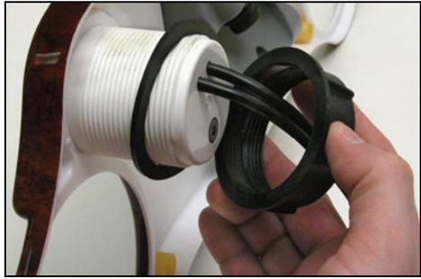
**Insert gauge through the hole in the front side of the dash (left). Slide the rubber gasket over the cables, followed by the plastic collar (right).** Slide the gasket forward so it is flush with the back of the dash, then screw on the mounting collar, turning it until it is snug against the gasket and the back of the dash.
