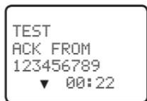
1. When you receive notification of a DSC TEST reply, press any key to cancel the alert.
