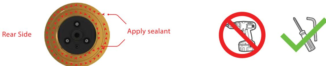
**Note: Do not use an alcohol-based solvent as this may have an adverse effect on the sealant**
