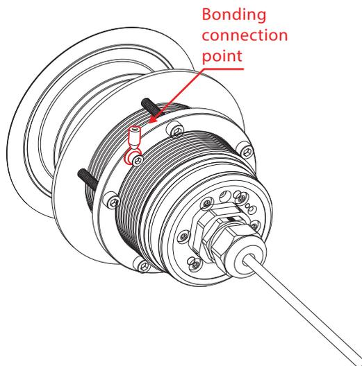
Metal Hull - isolation Sleeve
