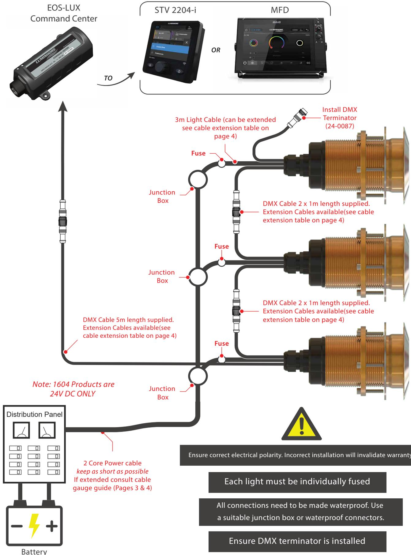
It is important to use the correct cable gauge for the installation. This can be split into two sections; Power source to Junction box and Junction box to each light.
