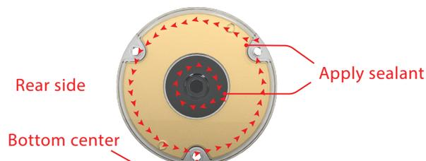
4. Apply a continuous thick bead of sealant to the back of the light, making sure the recess on the outer edge is slightly overfilled. Also apply a bead of sealant around the cable gland. Refer to image above.
