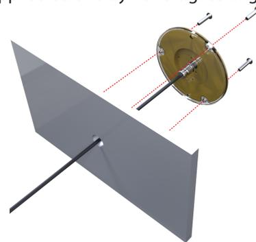
**IMPORTANT: Do Not Over Tighten. Do Not Use Power Tools to tighten screws.**
