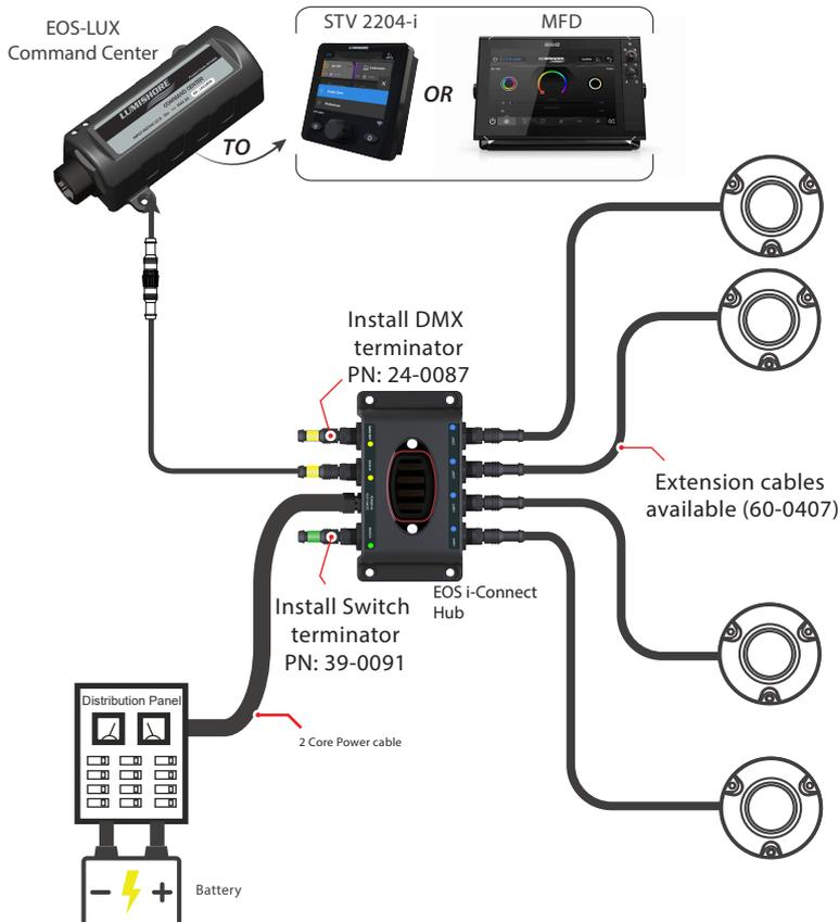
Note: Up to 4 hubs can be connected together. All they need is power connected, and a DMX Extension cable run between the hubs (see "Connecting additional hubs" section).
