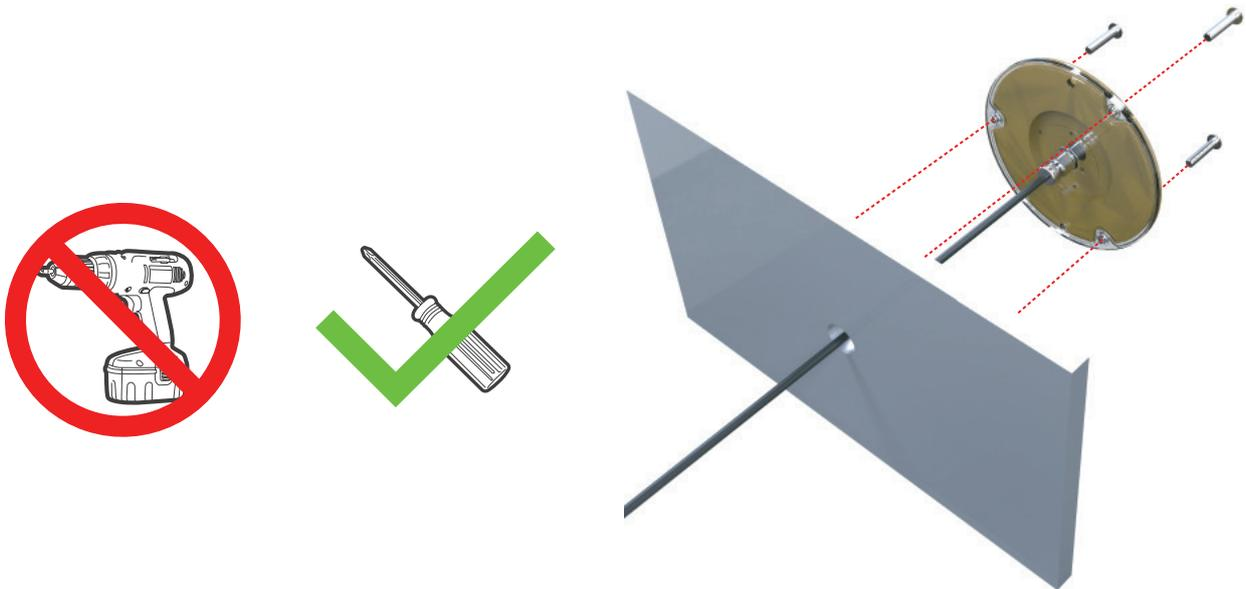
**IMPORTANT: Do not over tighten. Do not use power tools to tighten screws.**
