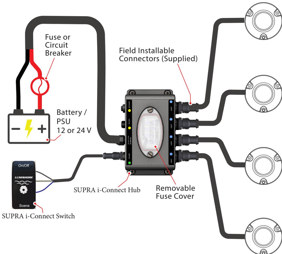
Note: Four hubs can be connected together. All they need is power connected, and a pre-moulded data cable run between the hubs (see connecting multiple hubs section for wiring diagram).
