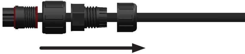
8. Wire the connector as shown below. TAKE CARE to secure the wires well with the grub screws. Check for any stray strands that could short to the other pins before fitting the strain relief and gland nut.
