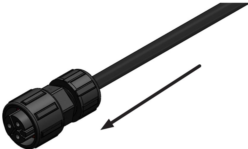
9. Fit and tighten the strain relief and gland nut onto the connector. Plug into the hub, taking care to orient the key correctly. Tighten the cap to make the waterproof seal.
