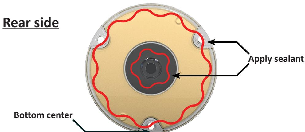
4. Apply a continuous thick bead of sealant to the back of the light, making sure the recess on the outer edge is slightly overfilled. Also apply a bead of sealant around the cable gland. Refer to image above.
