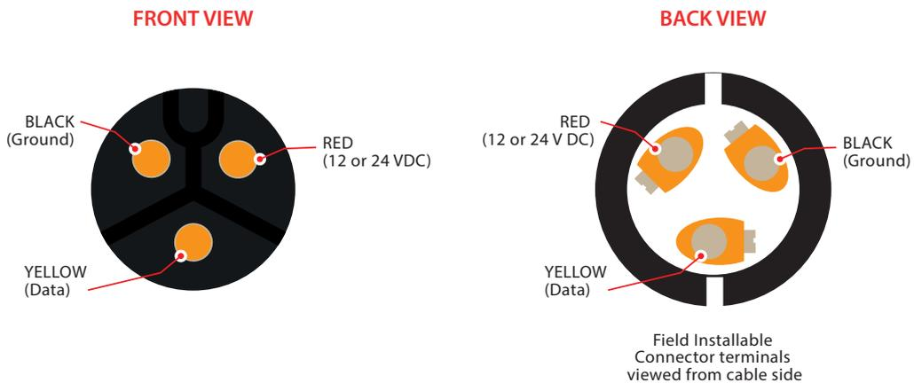
**Note: Check the wiring is correct before connecting to the hub. Incorrect wiring can damage the light.**
