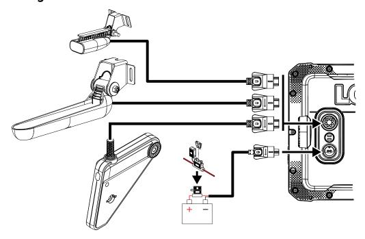
Connect a SplitShot $^{\text{\tiny{M}}}$ , TripleShot, or Eagle Eye $^{\text{\tiny{M}}}$  transducer. Refer to included transducer installation information.
