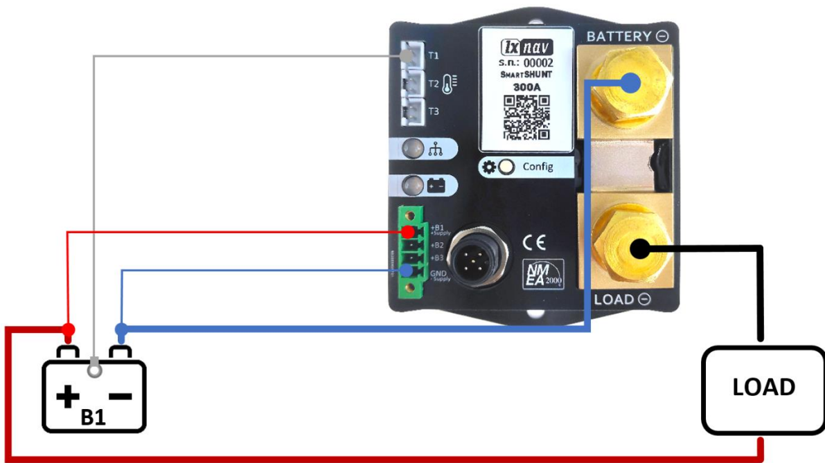
Figure 11: Wiring diagram for 1S Battery (e.g. 12V)
