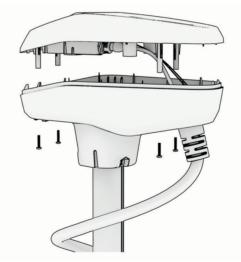
You should place these screws in a safe place, because you must use them to close the shaft cap.
