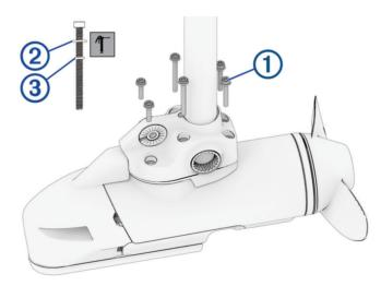
4 Using the grease packet included in the kit, apply grease to the 4.75 mm  $(^{3}/_{16} \text{ in.})$  O-ring on each bolt. Avoid getting grease on the bolt threads. 5 Apply a medium-strength thread-locking compound (not included) such as LOCTITE<sup>®</sup> 243<sup>™</sup> to the threads in the six threaded holes on the top of the propeller drive motor.
