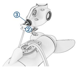
3 Straighten the cables at the top of the shaft, and slowly pull the propeller drive motor away from the shaft base until you can see the power and data cables ④ connected to the propeller drive motor.
