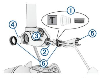
4 Using the included grommet nut wrench (5), tighten the grommet nuts (6).
