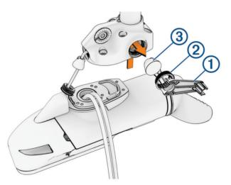
2 Push out the grommets ③ from the inside of the downshaft adapter.
