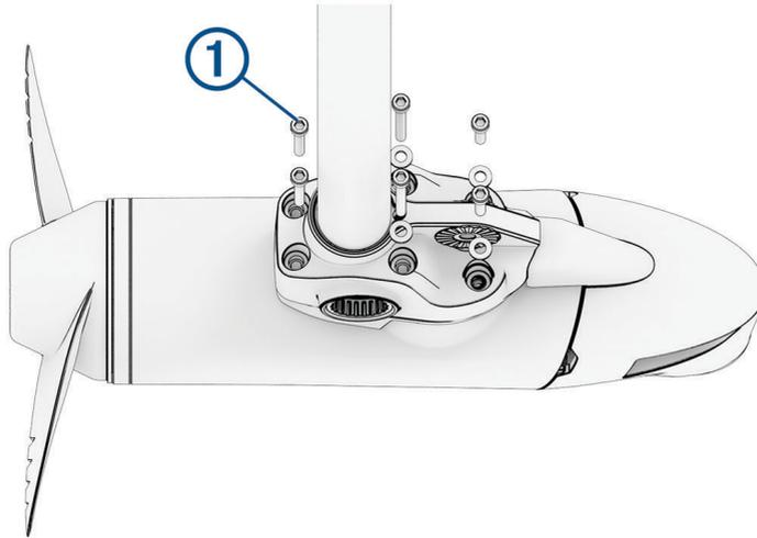
You should dispose of these six screws. New screws, washers, and O-rings are provided in the kit.
