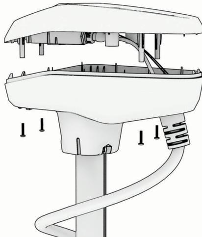
You should place these screws in a safe place, because you must use them to close the shaft cap.
